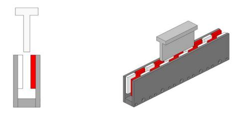
Figure 1: Brake is Completely Disengaged.
